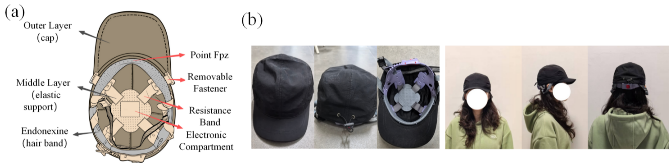
Figure 6: Structure Design of the Multi-Layer Cap.(a) Three-layer structure assembly diagram; (b) Final wearing appearance.
