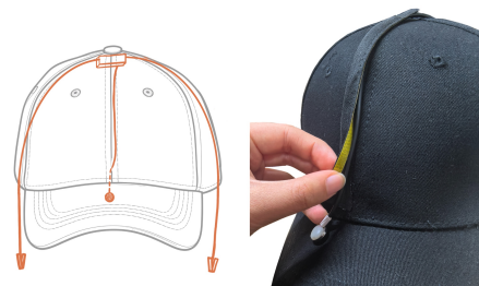
Figure 5: Signal Wires Layout and Channel Design
