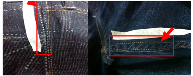
Figure 3: The bright line at the seam is not straight.
