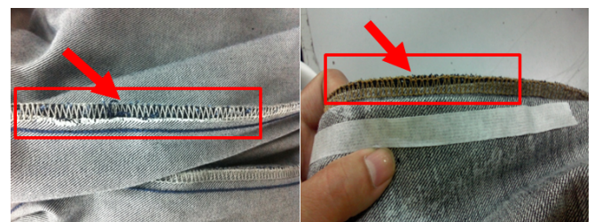
Figure 12: Two uneven pieces of the three-line overlock
