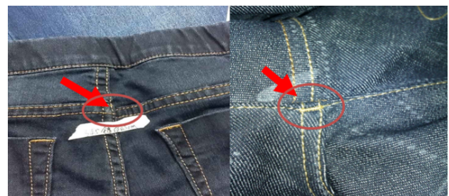
Figure 16: Severe misalignment of cross-alignment points
