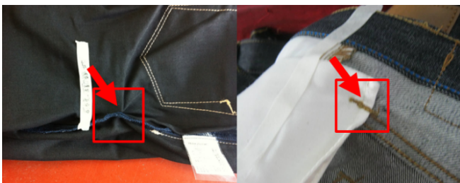
Figure 7: Misstitching to other locations of the sewing material.
